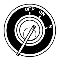
During engine operation, do not turn the key to "S" position. This may damage the starter motor.
